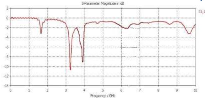
Figure 4. Return loss in db vs Resonating frequency for circular patch antenna with U-slot
